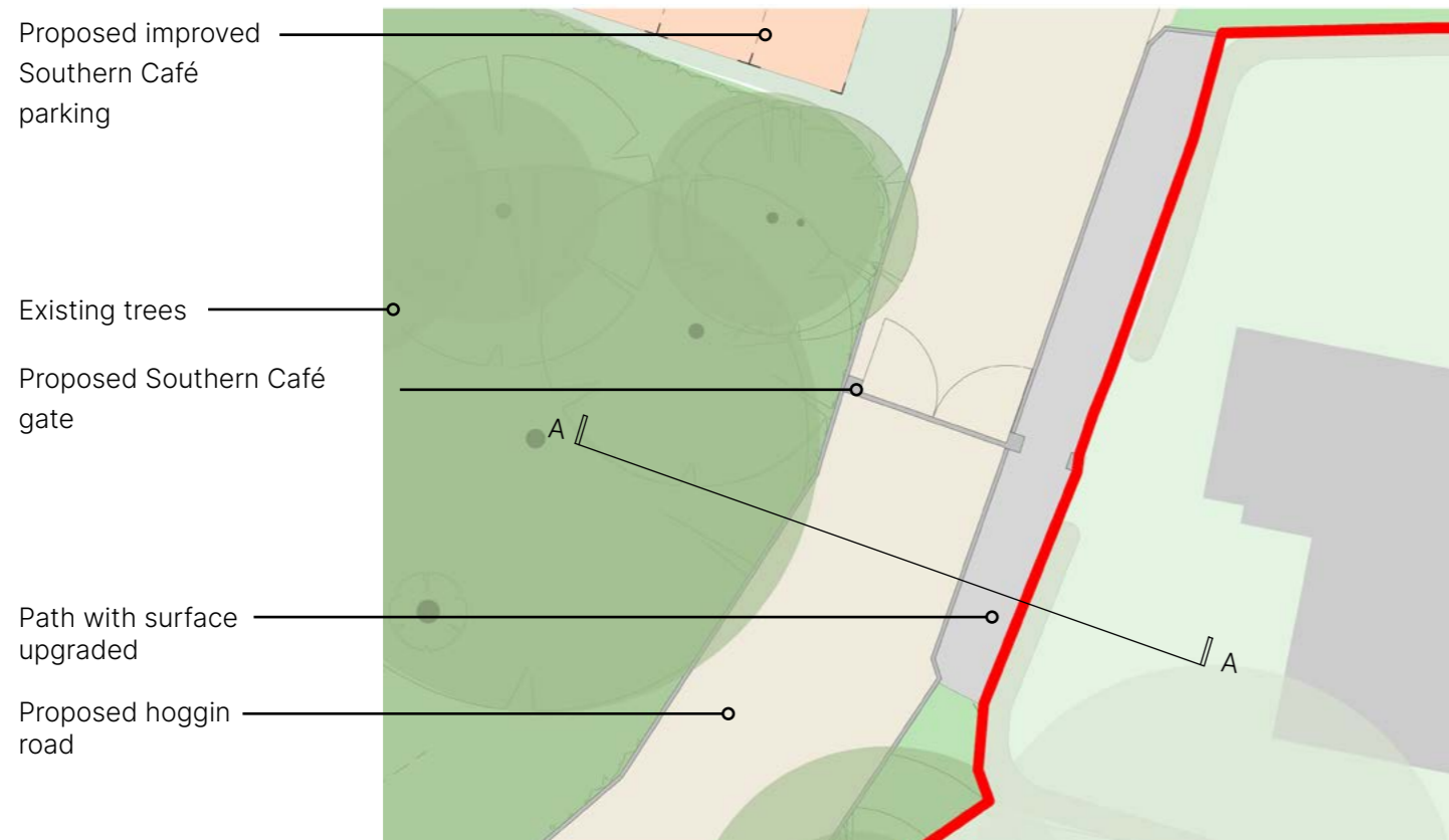
FIGURE 142. Proposed Gate Plan
